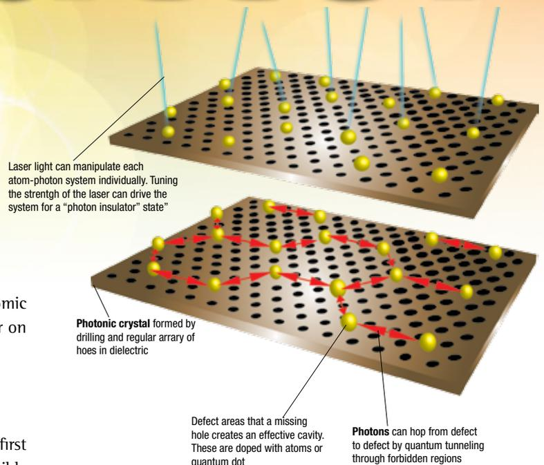
Figure 1: A quantum simulator made out of photons. Light is trapped in the cavity defects—circular yellow areas— which are doped with atoms. A crystal of light is thus formed that can simulate (mimick) the behaviour of complex real crystals made of atoms. By tuning external fields the properties of various complex phases of matter like insulators, and superconductors, can be probed and understood with high efficiency.
